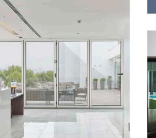
**Bi-fold system** with Thermal break specially for enclosing large gaps with the most avant-garde aesthetic. It has a range variety of compositions up to 14 sashes in outwards & inwards openings. Allows to inlay bottom frame leaving threshold completely accessible.
